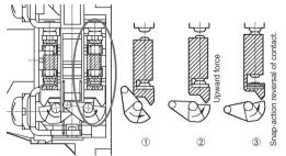
As seen above, the cam forces the N.C. contact up from the bottom, even if there is fusing of the contacts.
