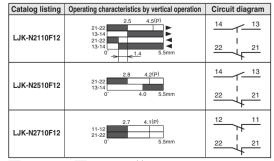
: Contacts closed : Contacts open (P): Min. travel to positive opening position
