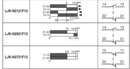
: Contacts closed :: Contacts open (P): Min. travel to positive opening position
