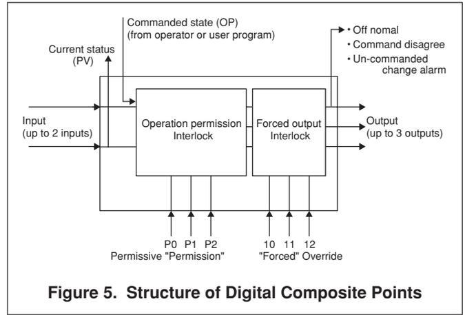
**Figure 5. Structure of Digital Composite Points**
