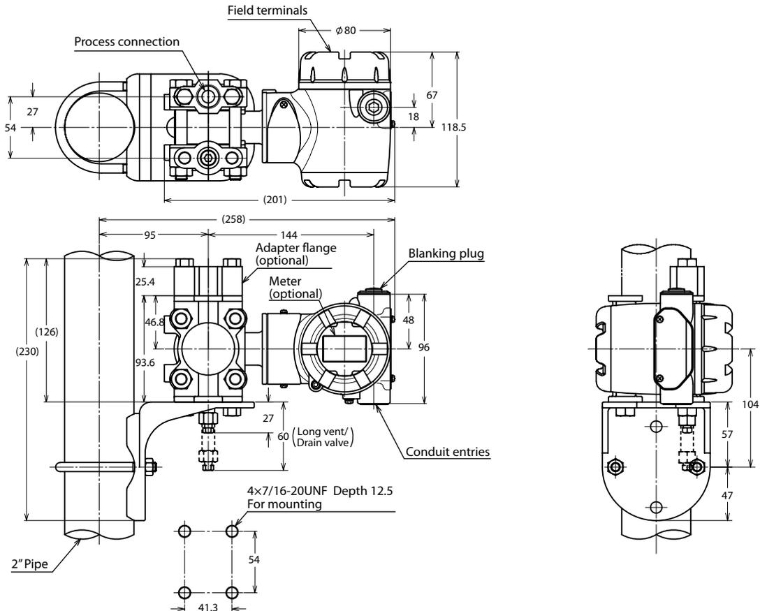
**Model GTX30A/60A (Material (center body): ASTM B575, Tantalum, 316L SST)**
