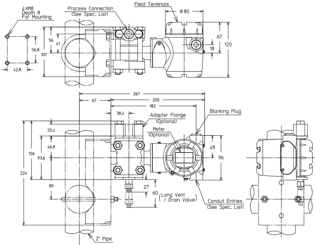
**Model GTX30A/60A (Material (Meter body cover, Vent/Drain plugs): PVC)**
