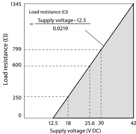
**Figure 3. Supply voltage vs. load resistance characteristics**
