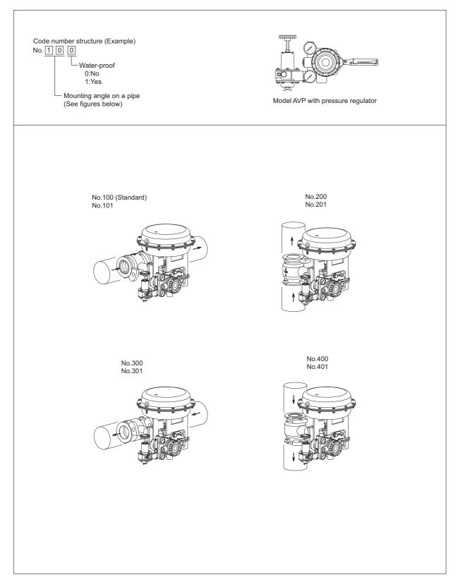
Figure 7 Mounting position of valve on process pipes (Applicable to model AVP positioner with pressure regulator)
