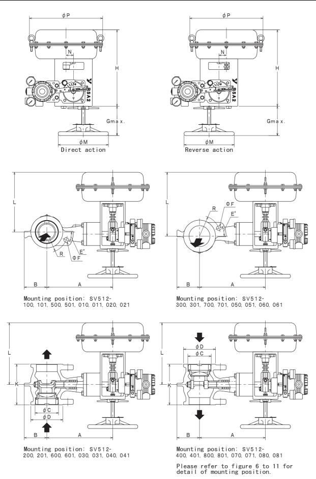
Figure 3 Face-to-face and external dimension in wafer connection
