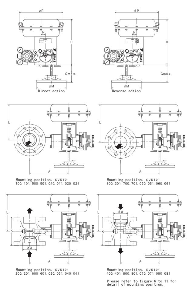
Figure 4 Face-to-face and external dimension in flange connection
