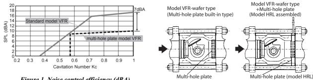
Figure 1 Noise control efficiency (dBA)
