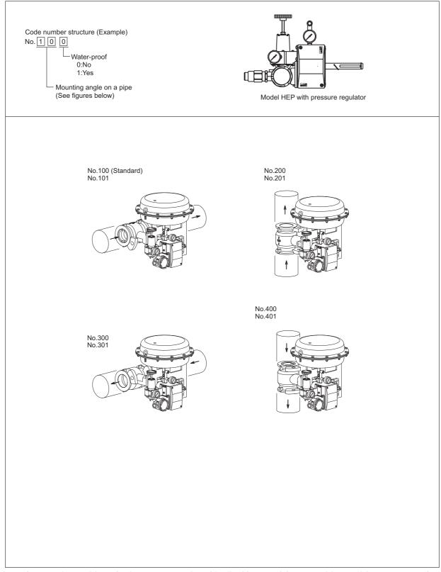
Figure 9 Mounting position of valve on process pipes (Applicable to model HEP positioner with pressure regulator)
