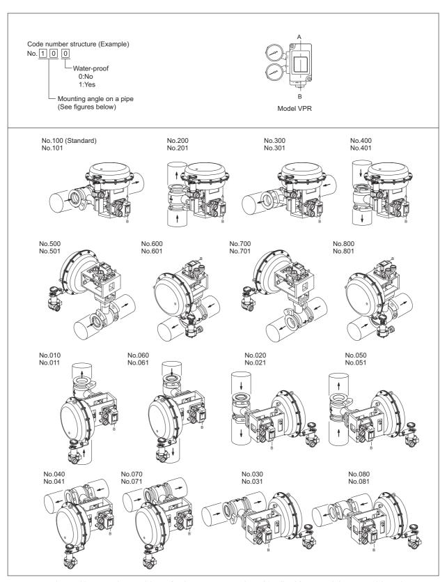
Figure 11 Mounting position of valve on process pipes (Applicable to model VPR positioner)
