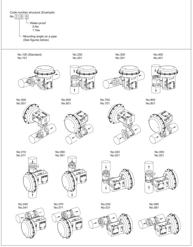
Figure 6 Mounting position of valve on process pipes (Applicable to non-positioner case)
