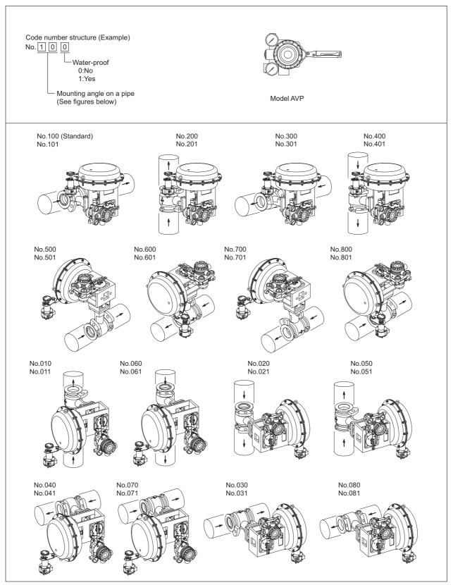
Figure 8 Mounting position of valve on process pipes (Applicable to model AVP positioner)
