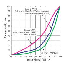
a. Flow characteristics of valve b. Positioner cam/unit characteristics
