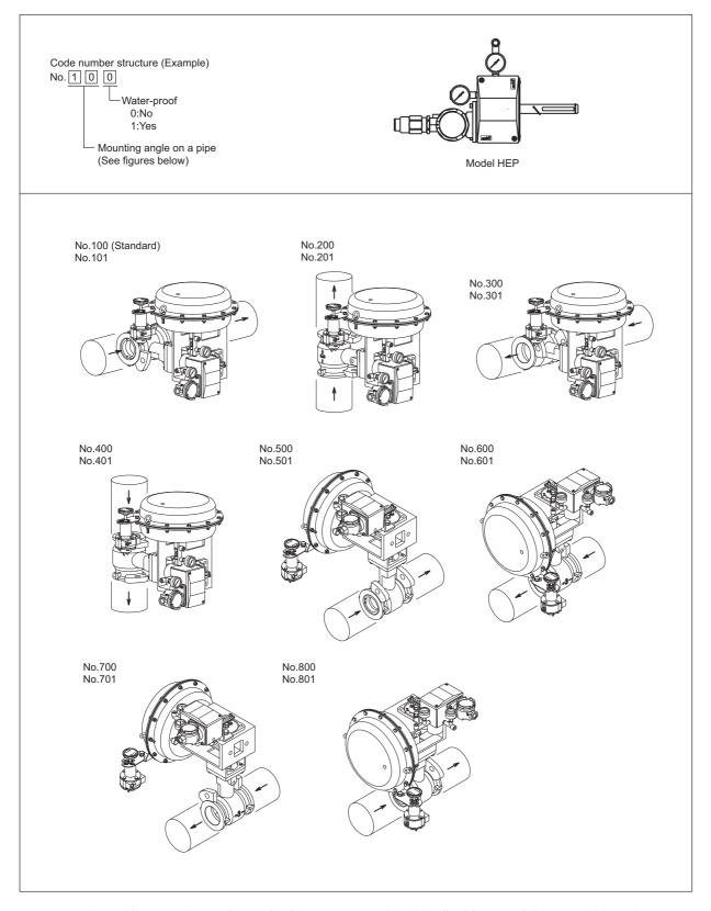
Figure 10 Mounting position of valve on process pipes (Applicable to model HEP positioner)
