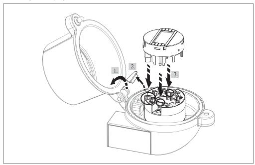
Fig 4-2. Mounting the display
