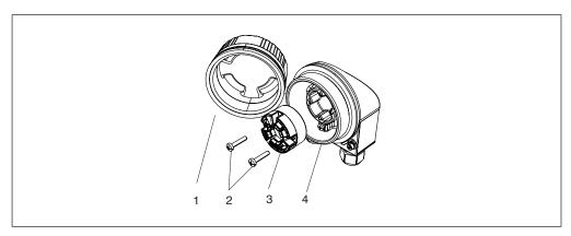
Fig 4-1. Head transmitter mounting
