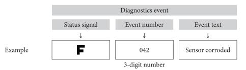
If two or more diagnostics events are pending simultaneously, only the message with the highest priority is shown. Additional pending diagnostic messages are shown in the ""Diagnostics list" submenu", (Refer to page 92).
