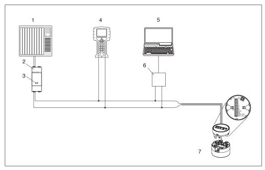
Fig 6-1. Operating options of the head transmitter
