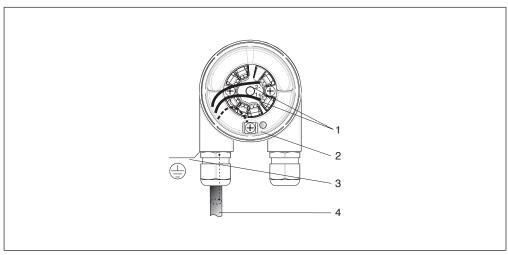
Fig 5-2. Connecting the signal cables and power supply
