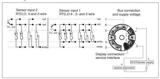
Fig 5-1. Wiring the head transmitter
