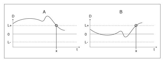
Fig 13-1. Drift/difference mode
