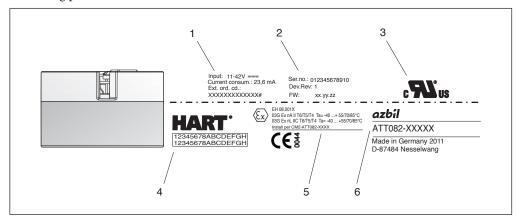
Fig 3-1. Nameplate of the head transmitter (example, Ex version)
