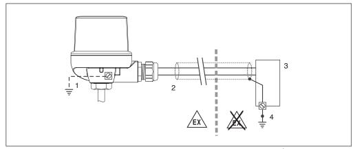
Fig 5-3. Shielding and grounding the signal cable at one end with HART communication
