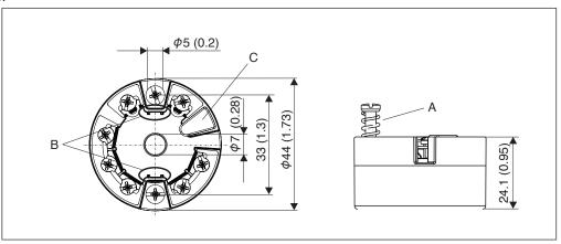
Fig 12-1. Version with screw terminals
