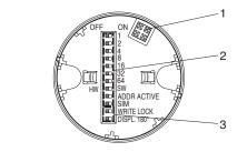
Fig 6-3. Hardware settings via DIP switches
