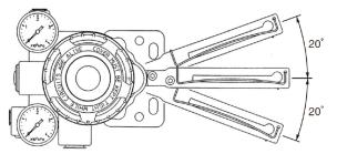
Figure 2-4. Feedback Lever Operating Angle
