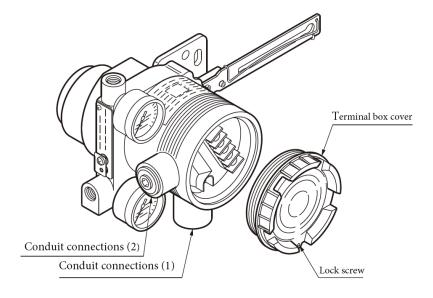
Figure 1-6. Structure of Terminal Box
