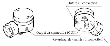
Figure 2-9. Reversing Relay Standalone View
