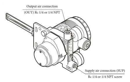
Figure 2-7. Air Piping Connection
