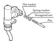
Attachment of feedback lever (pin)
