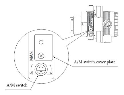
Figure 5-5. A/M Switch Structure
