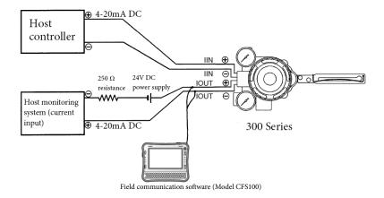
Figure 4-3. Using the Travel Transmission Function (Model AVP301/201)
