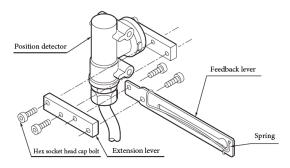
Attachment of Extension Lever and Feedback Lever
