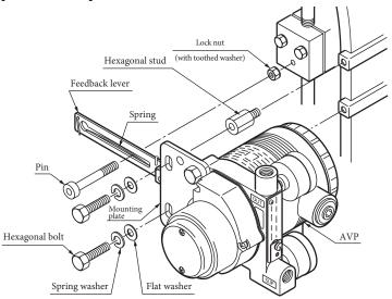
Figure 2-1-1. Mounting the Device on an HA1 Actuator
