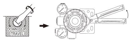
Figure 3-2-1. Adjusting the Lever in the Upward Direction
