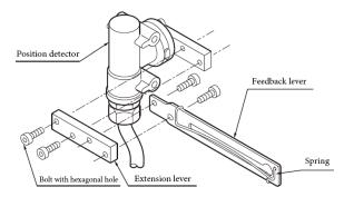
Attachment of Extension Lever and Feedback Lever
