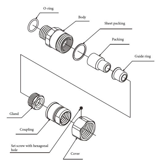
Figure 2-25. Flameproof Cable Gland Exploded View
