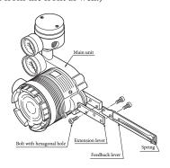
Attachment of Extension Lever and Feedback Lever
