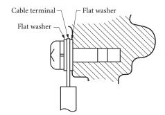
Figure 2-13. Connection to the external ground terminal
