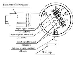
Figure 2-12. Terminal Block of Terminal Box
