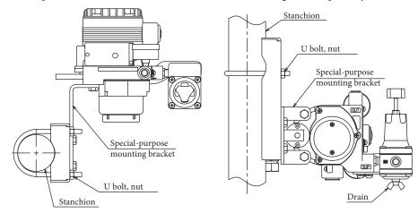
Figure 2-21. Positioner Body Installation
