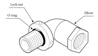
Figure 2-26. Explosion-proof Elbow Structure
