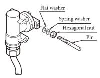
Attachment of Feedback Lever (Pin)
