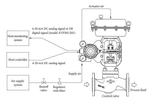
Figure 1-1. Control System Overview Diagram
