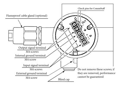
Figure 1-7. Terminal Block of Terminal Box
