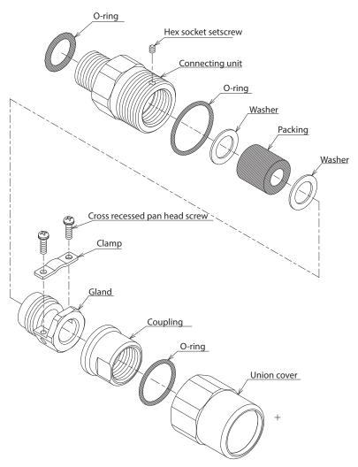
Figure 2-23. Flameproof Cable Gland Exploded View
