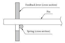
Figure 2-2. Attachment of Feedback Lever and Feedback Pin
