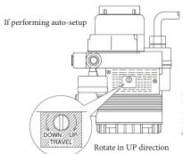
Note: When closing the valve of the single-acting type device with the lever in the upward direction, first set it to reverse close.
