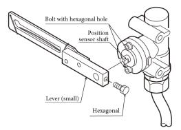
Figure 2-20. Valve Travel Detector
