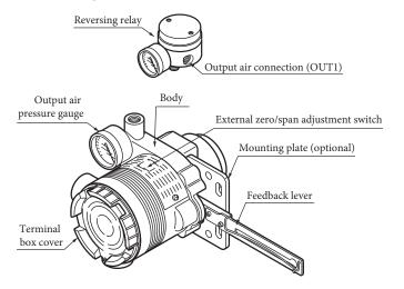
Figure 1-5-1. Body Structure (Front)
