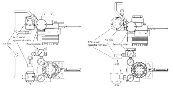
Figure 2-10-1. Air Pipe to Reversing Relay when Model RA1B Is Installed Integrally
