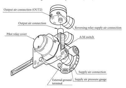
Figure 1-5-2. Body Structure (Rear)
