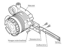
Attachment of Extension Lever and Feedback Lever
