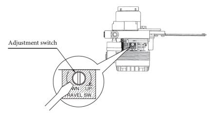
Figure 3-1. External Zero/Span Adjustment Unit Structure
