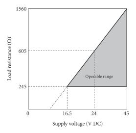
Figure 2-16. Supply Voltage and Load Resistance Characteristics
