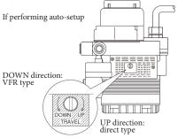
Note: When closing the valve of the single-acting type device with the lever in the upward direction, first set it to reverse close.
