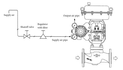
Figure 2-6. Air Supply System
