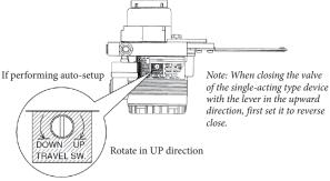
External zero/span adjustment switch
