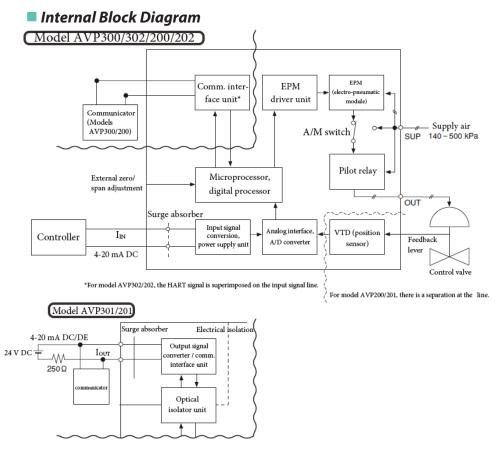
Figure 5-6. Internal Block Diagram
