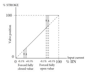
Figure 4-5. Forced Fully Open/Closed Settings
