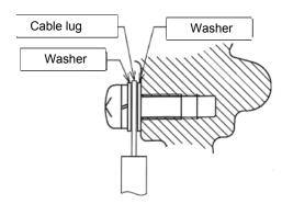
Figure 2-17. Connection of External Grounding Terminal
