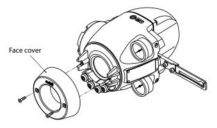
Figure 6-6. Removal of face cover
