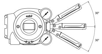
Figure 2-8. Operation Angle of Feedback Lever
