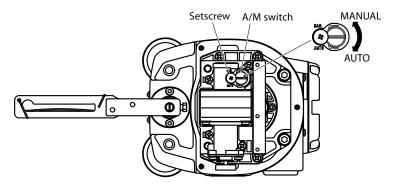
Figure 6-1. Structure of A/M Switch
