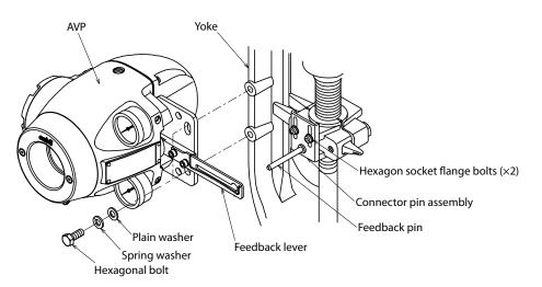
Figure 2-3. Mounting Procedure for Direct-Acting Actuator HA2 to 4, PSA1 to 4, 6, VA1 to 6 from Azbil Corporation
