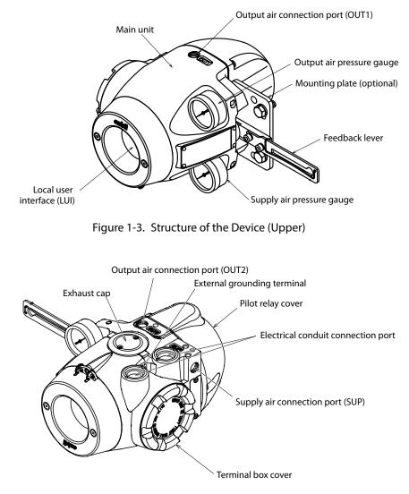
Figure 1-4. Structure of the Device (Lower)
