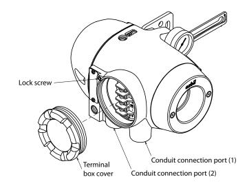
Figure 1-5. Structure of Terminal Box
