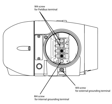
Figure 1-6. Terminal Block in the Terminal Box
