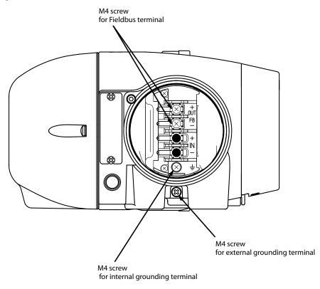
Figure 2-16. Terminal Block in the Terminal Box
