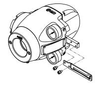
Figure 2-1. Mounting Procedure for Feedback Lever
