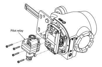
Figure 6-9. Removal of pilot relay
