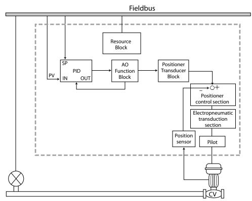
Figure 1-2. Operation Block Diagram (AVP703)
