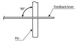
Figure 2-7. Angle between Feedback Lever and Pin
