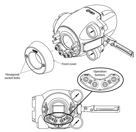
Figure 3-1. LUI Structure with the Front Cover Removed
