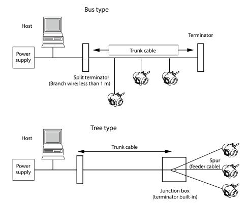
Figure 2-18. How to Install Fieldbus Networks
