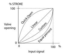
Figure 4-1. Concept of Flow Amount Characteristics
