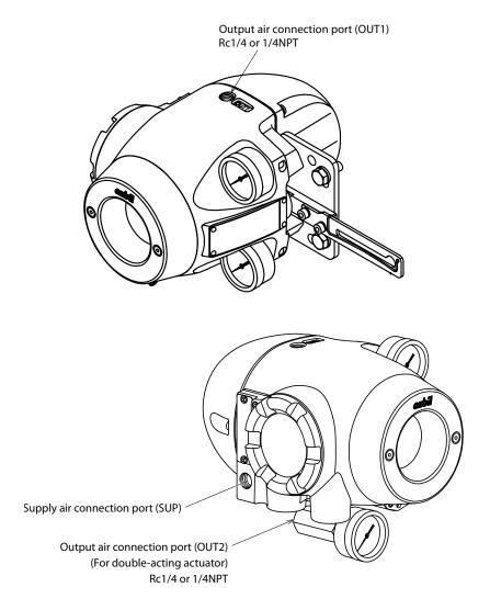
Figure 2-15. Pneumatic Piping Connection
