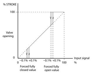
Figure 4-2. Forced Fully Open and Closed Values
