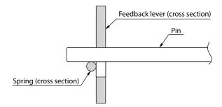
Figure 2-6. Connection of Feedback Lever and Feedback Pin
