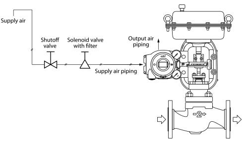
Figure 2-14. Air Supply System
