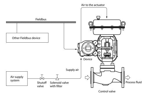
Figure 1-1. Concept Diagram of the 700 Series Control System
