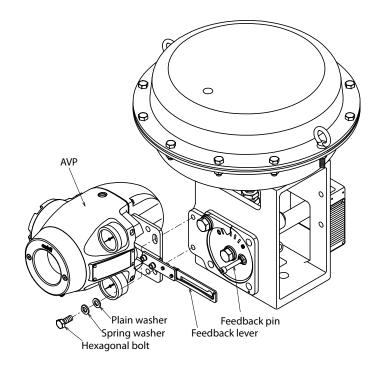
Figure 2-4. Mounting Procedure for RSA1, 2, VR3 Actuator from Azbil Corporation
