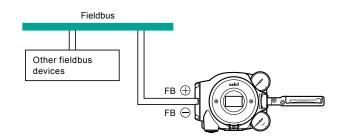
Figure 2. Wiring example of AVP703
