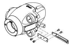
Figure 2-2. Mounting Procedure for Extension Lever
