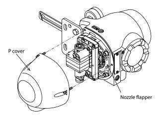
Figure 6-8. Removal of P cover
