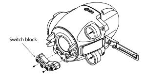
Figure 6-7. Removal of switch block
