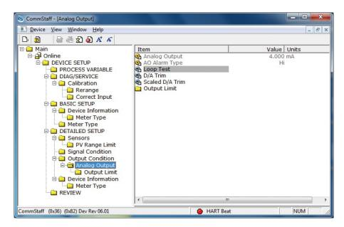
Double-clicking Loop Test displays the following screen.
