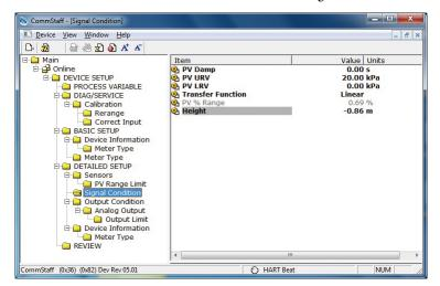
Select DEVICE SETUP  $\rightarrow$  DETAILED SETUP  $\rightarrow$  Signal Condition  $\rightarrow$  Height.
