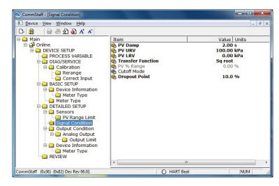
Linear: Linear output Sq root: Square root output
