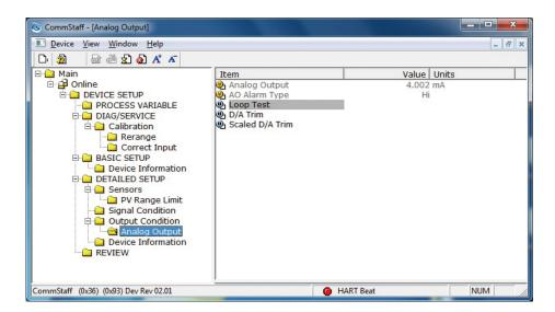
Double-clicking Loop Test displays the following screen.
