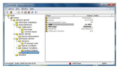
Double-clicking Tag displays the settings screen. On this screen, set the Tag and click the Set button. The tag is highlighted in yellow. Click the Send button to send the new Tag to the device.
