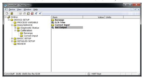
A warning that the loop should be switched from automatic control to manual mode is displayed (WARNING: Loop should be removed from automatic control). After switching to manual mode, click OK.
