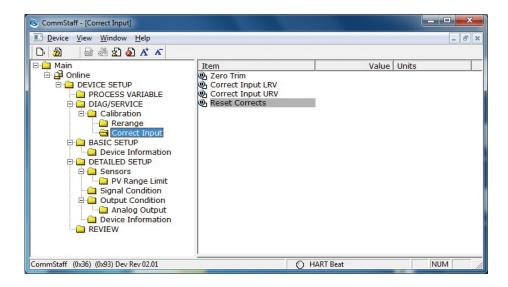
CAUTION: If this operation is performed while the device process is under automatic control, outputs may fluctuate, making device operation dangerous. Before performing this operation, make sure that you switch the process control loop to manual control.
