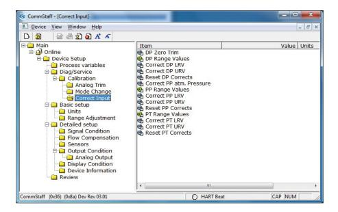
Select [Device Setup]  $\rightarrow$  [Diag/Service]  $\rightarrow$  [Calibration]  $\rightarrow$  [Correct Input].
