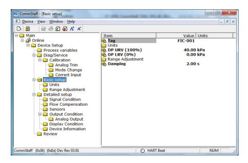
Double-clicking Tag displays the settings screen. On this screen, set the Tag and click the Set button. The tag is highlighted in yellow. Click the Send button to send the new Tag to the transmitter.
