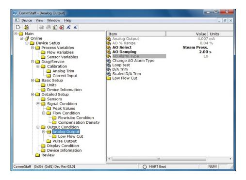
To change the direction of burnout, select [Device Setup]  $\rightarrow$  [Detailed Setup]  $\rightarrow$  [Output Condition]  $\rightarrow$  [Analog Output]  $\rightarrow$  [Change AO Alarm Type].
