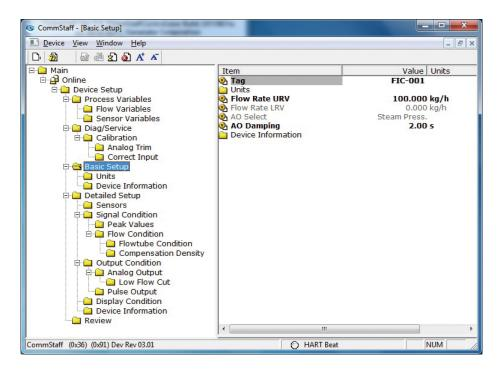
Double-clicking Tag displays the settings screen. On this screen, set the Tag and click the Set button. The tag is highlighted in yellow. Click the Send button to send the new Tag to the transmitter.
