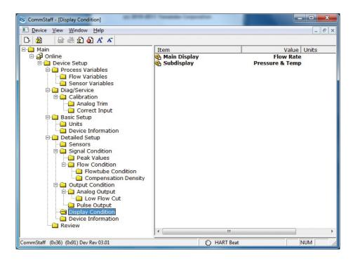
The Main Display can be selected to show either Total Flow or Flow Rate.
