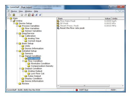
To reset Flow Rate Peak to 0, select [Reset the flow rate peak].
