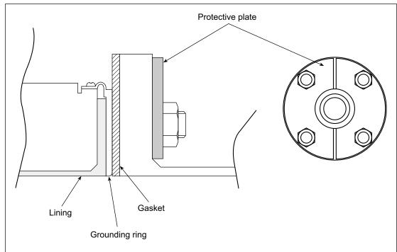
Figure 2-16 Installation on a PVC pipe using SUS grounding ring material and a protective plate
