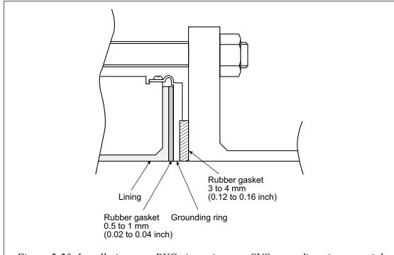
Figure 2-20 Installation on a PVC pipe using non-SUS grounding ring material with rubber gaskets
