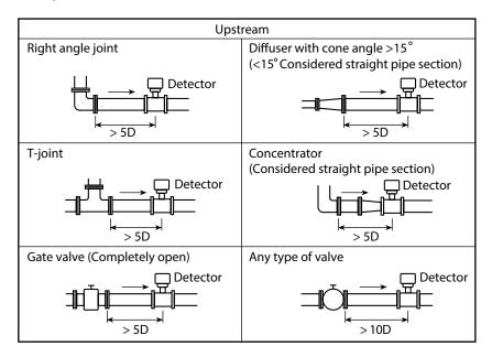
Figure 2-2 Straight pipe section on upstream side of detector
