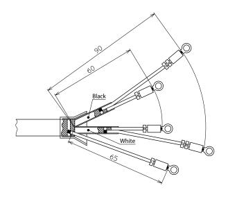
Figure 2-47 Terminal connections
