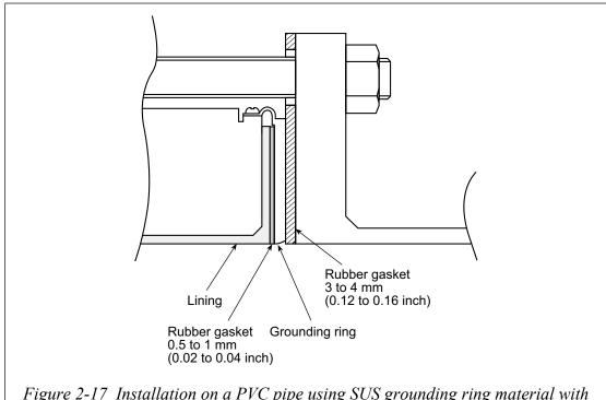
Figure 2-17 Installation on a PVC pipe using SUS grounding ring material with rubber gaskets (Not recommended)
