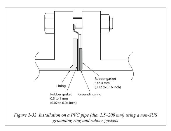
(5) Fasten the bolts with a torque that provides a leakproof joint.
