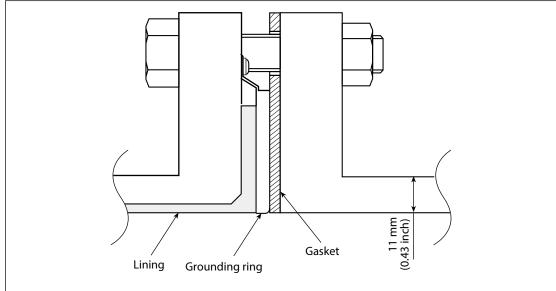
Figure 2-27 Installation on a PVC pipe (SUS ring & pipe dia. 2.5–1100 mm, or non-SUS ring & pipe dia. 250–1100 mm)
