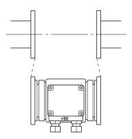
Figure 2-8 Unacceptable placement of detector between flanges
