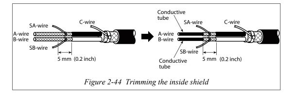
(9) Peel off the conductive tube (black) completely up to the inside shield.
