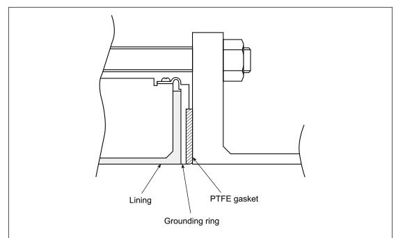
Figure 2-12 Installation on a metal pipe using non-SUS grounding ring material and a specified torque
