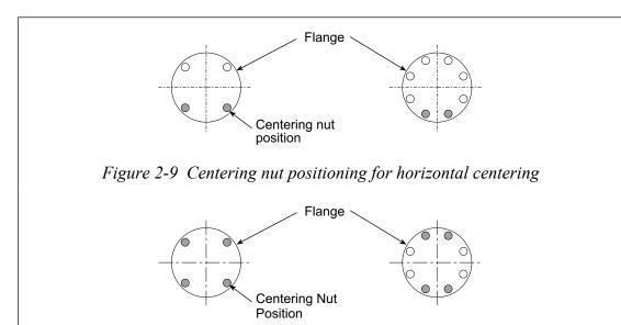
Figure 2-10 Centering nut positioning for vertical centering
