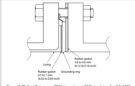
Figure 2-29 Installation on a PVC pipe using an SUS ring (pipe dia. 2.5–1100 mm) or a non-SUS ring (pipe dia. 250–1100 mm) and rubber gaskets (not recommended)
