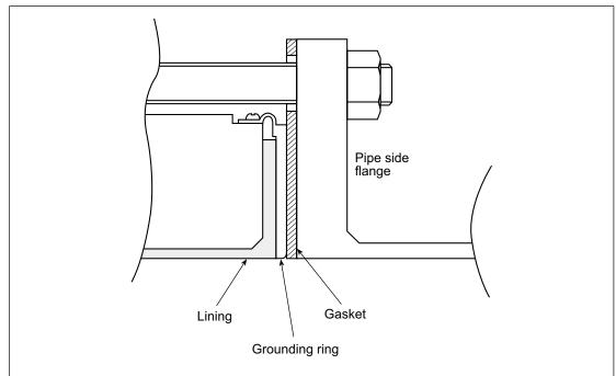
Figure 2-11 Installation on a metal pipe using SUS grounding ring material and a specified torque
