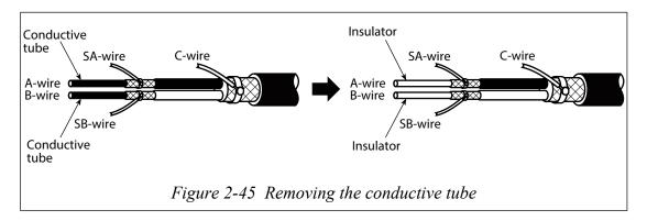
(10) Trim the insulator to within 5 mm (0.2 inch) from its end. Trim the other lead wires (soldered to the shield sections) to the specified lengths so that each conductive wire is exposed by 5 mm (0.2 inch).
