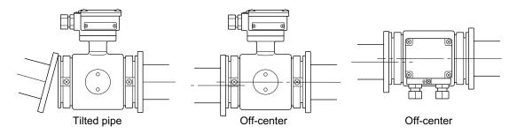
Figure 2-7 Unacceptable positioning
