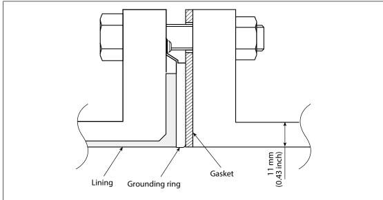
Figure 2-24 Installation on a metal pipe (SUS ring & pipe dia. 2.5–1100 mm, or non-SUS ring & pipe dia. 250–1100 mm)
