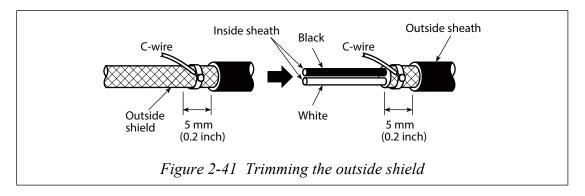
(5) Peel off the inside sheath so that a 15 mm (0.59 inch) section remains.
