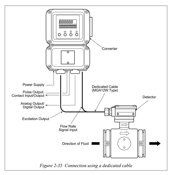
**~Note** Although the dedicated cable is shielded, install it away from any possible sources of noise, such as a large capacity transformer, motors, or motor power supplies.
