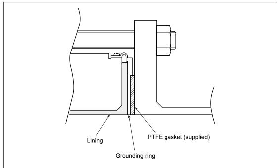
Figure 2-18 Installation on a PVC pipe using non-SUS grounding ring material
