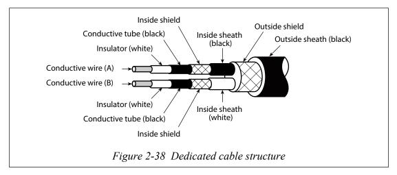
**Note** The conductive tubing (black) for conductive wires (A) and (B) is to be removed up to the end of the inside shield.
