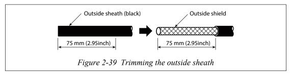
**Note** If the terminal of the converter is designed not to use a shield drive, remove the outside shield and skip to Step 4.
