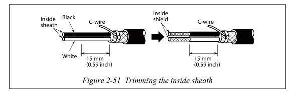
(6) Cut the inside shield off at a point 5 mm (0.2 inch) from the edge.
