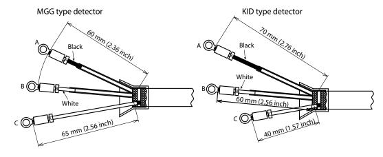
Figure 2-54 Terminal connections
