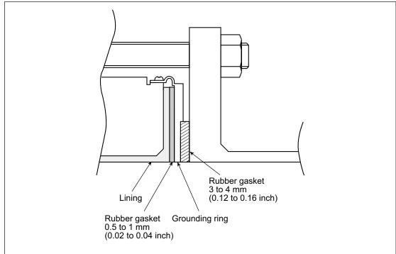
Figure 2-13 Installation on a metal pipe using non-SUS grounding ring material with rubber gaskets
