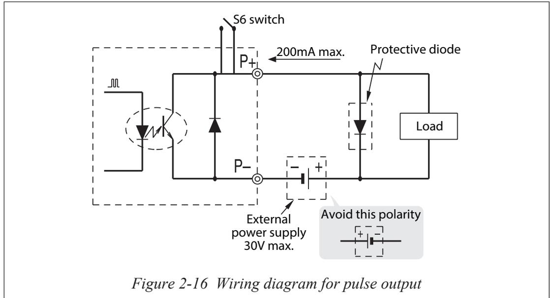
Figure 2-16 Wiring diagram for pulse output
