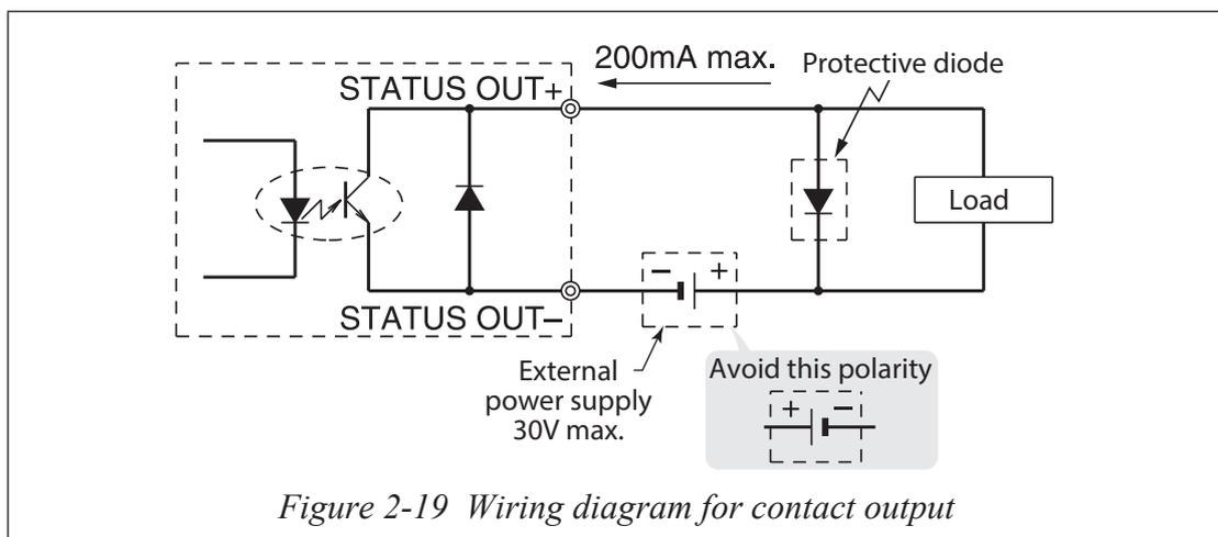
Figure 2-19 Wiring diagram for contact output
