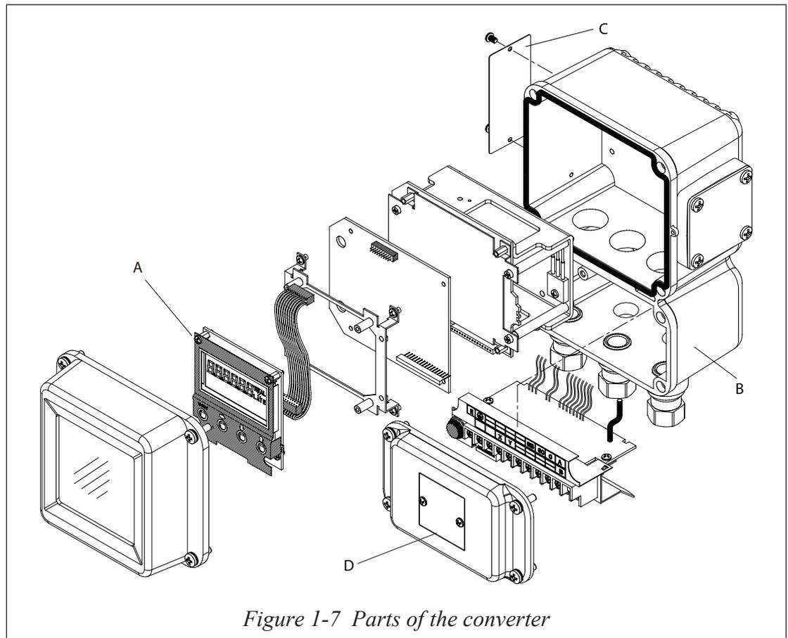
Figure 1-7 Parts of the converter
