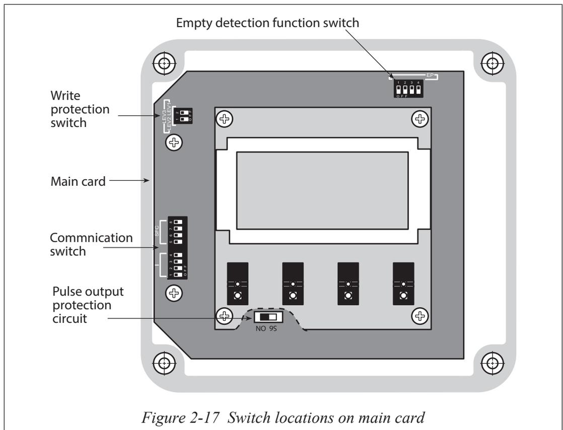
Figure 2-17 Switch locations on main card
