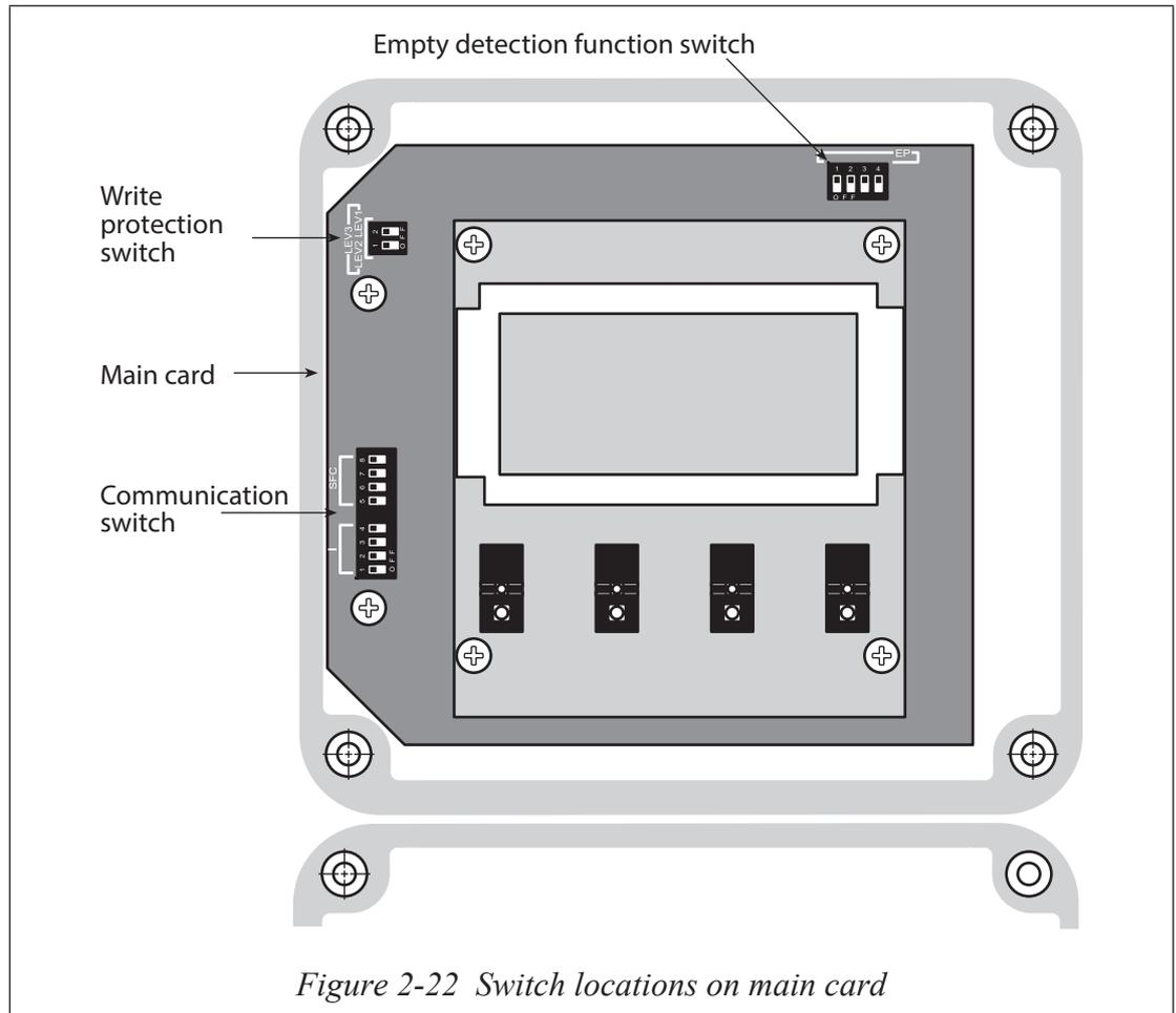
3. Make sure that position of the I switch (1-4) are ON and positions of the SFC switch (5-8) are OFF.
