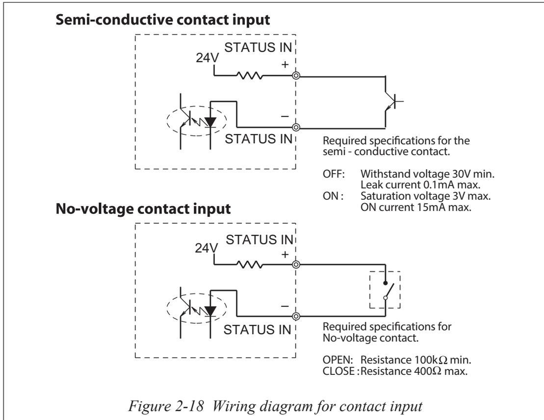
Figure 2-18 Wiring diagram for contact input
