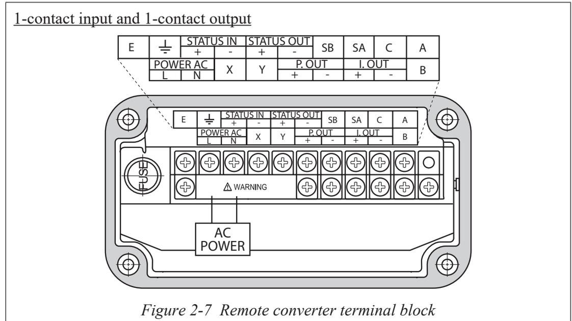
Figure 2-7 Remote converter terminal block
