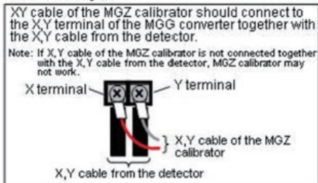
In case the X,Y cable from the detector is not connected together with the X,Y cable of the MGZ calibrator, upgrade the S/W version of MGZ from the current version to 1.7 or later version.
