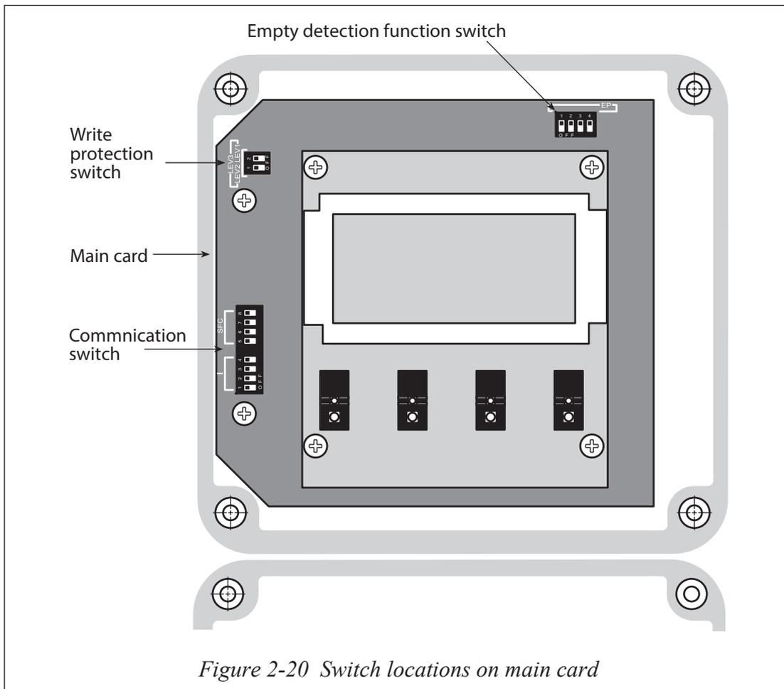
Figure 2-20 Switch locations on main card
