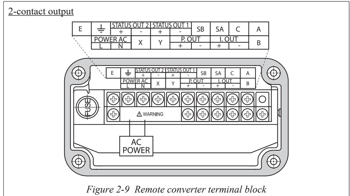
Figure 2-9 Remote converter terminal block
