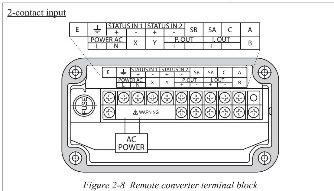
Figure 2-8 Remote converter terminal block
