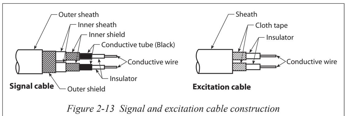
Figure 2-13 Signal and excitation cable construction
