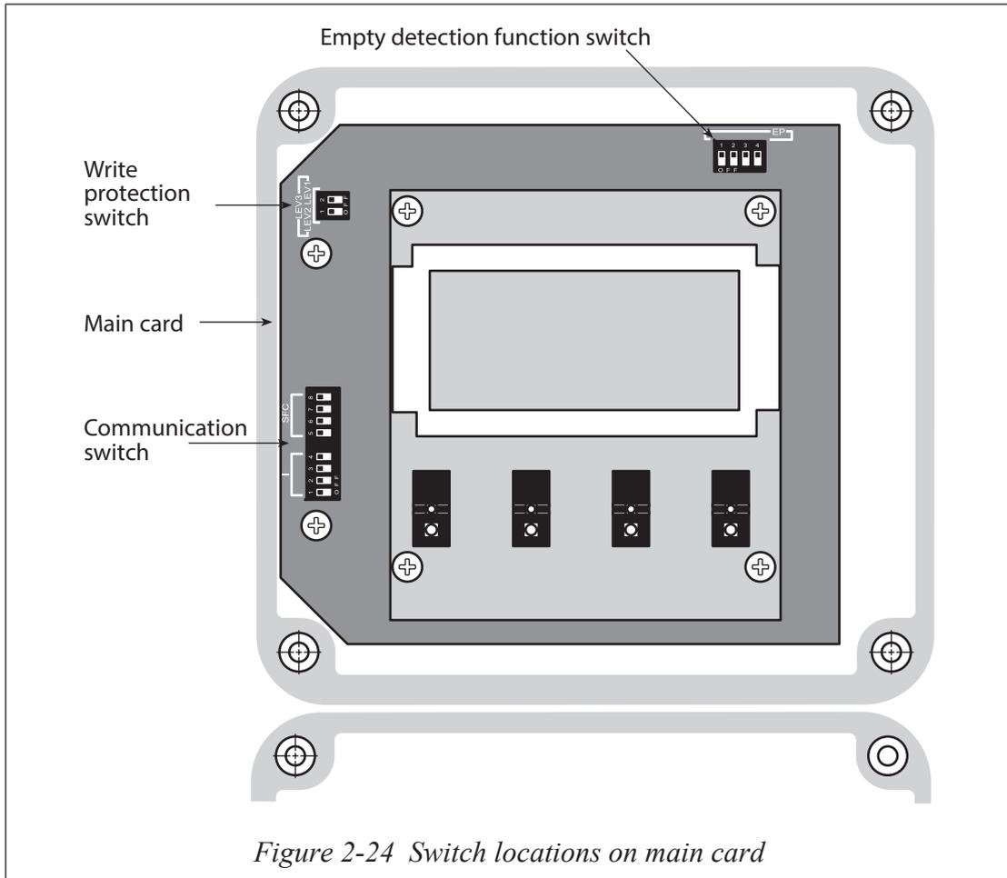
3. Set the empty detection function switch positions to the required setting.
