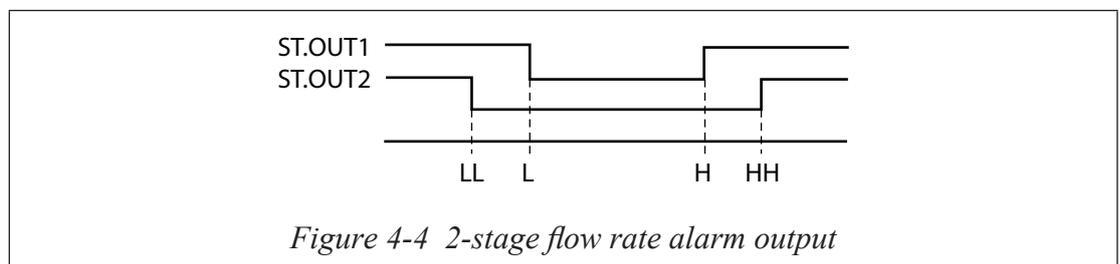
*Figure 4-4 2-stage flow rate alarm output*
