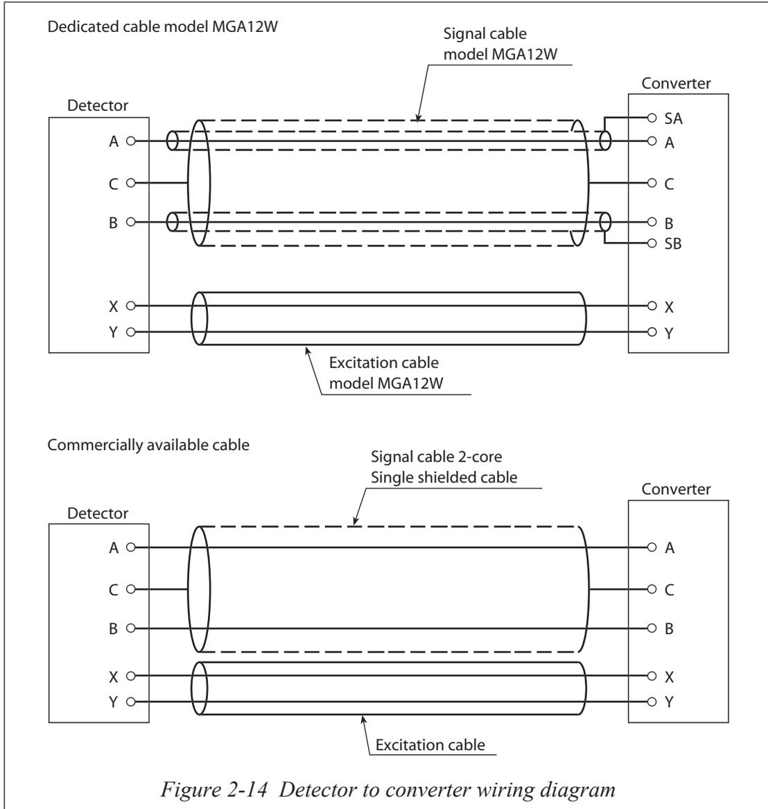
Figure 2-14 Detector to converter wiring diagram
