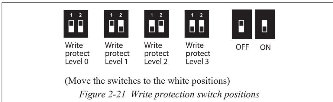
Figure 2-21 Write protection switch positions
