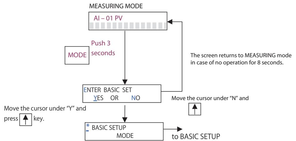
Figure1-7 How to enter BASIC SETUP
