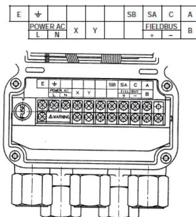
Figure 3-3 Terminal layout of remote transmitter
