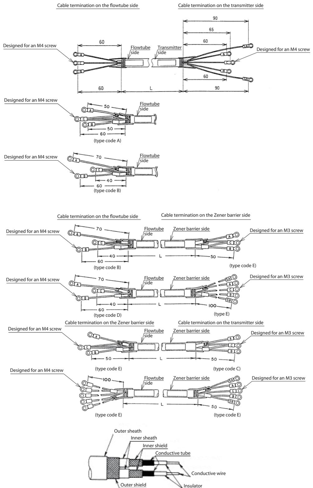
Note) Remove the conductive tubes (black) of conductive cables for terminals A and B up to the edges of the inner shields.
