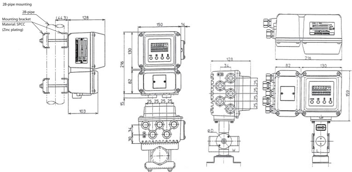
Figure3-2 2B-pipe mounting of transmitter and Integrated mounting
