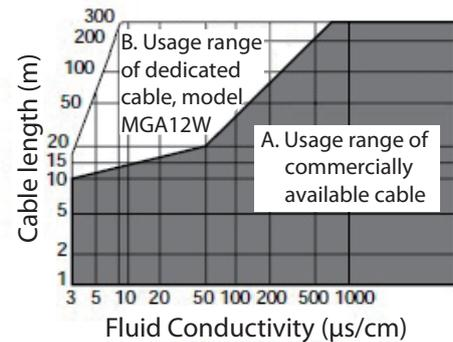
Figure3-4 Relationship between the fluid conductance and cable length
