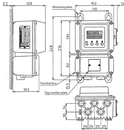
Figure3-1 Wall-mounting of transmitter
