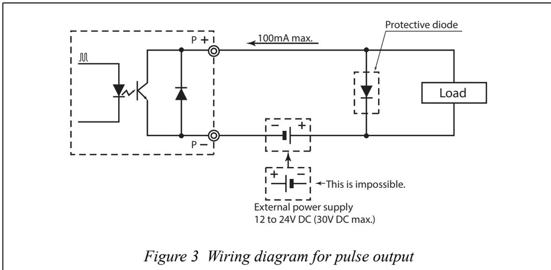
Figure 3 Wiring diagram for pulse output
