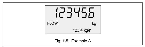
Main display:Cumulative flow = 123456 kgAuxiliary display:Instantaneous flow rate = 123.4 kg/hAnalog output:Instantaneous flow rate (FLOW)
