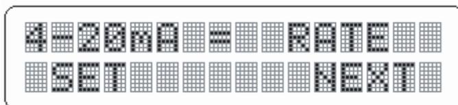
The 4-20 mA output can be allocated either the current flow rate or the temperature.
