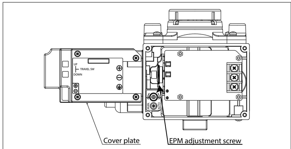
Fig. 5-5. EPM balance adjustment
