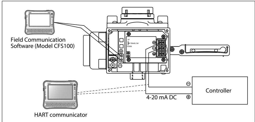
Fig. 1-3. System structure for model SVX102
