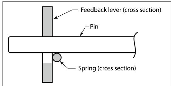
Fig. 2-4. Feedback pin and feedback lever connection
