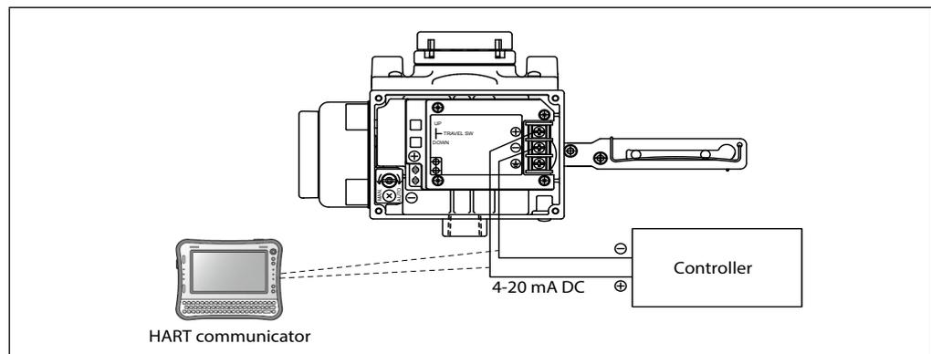
Fig. 4-1. Wiring of HART® Communication Tool (Model SVX102)
