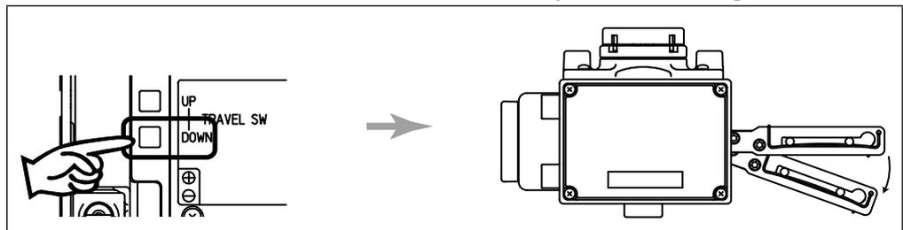
Fig. 3-3. Adjusting the lever in the downward direction
