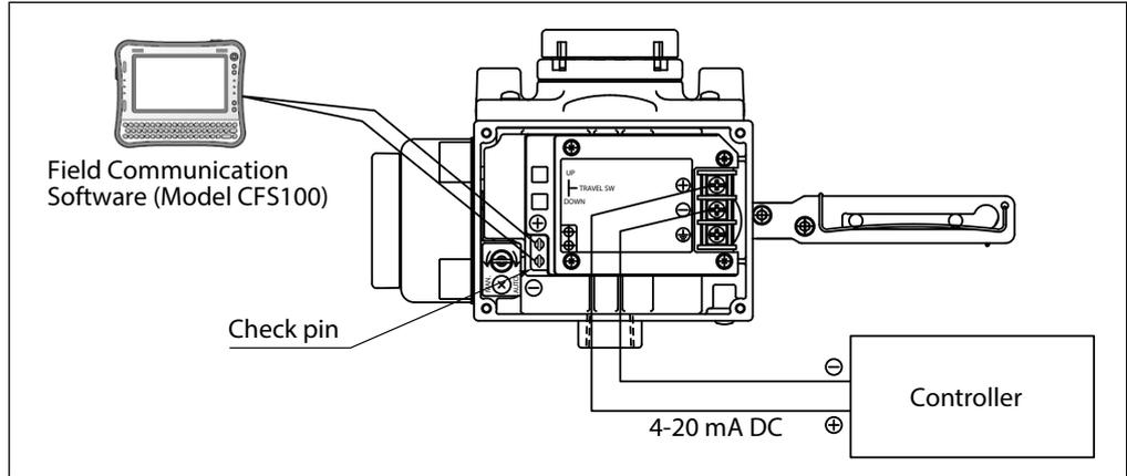
Fig. 1-2. System structure for model SVX100
