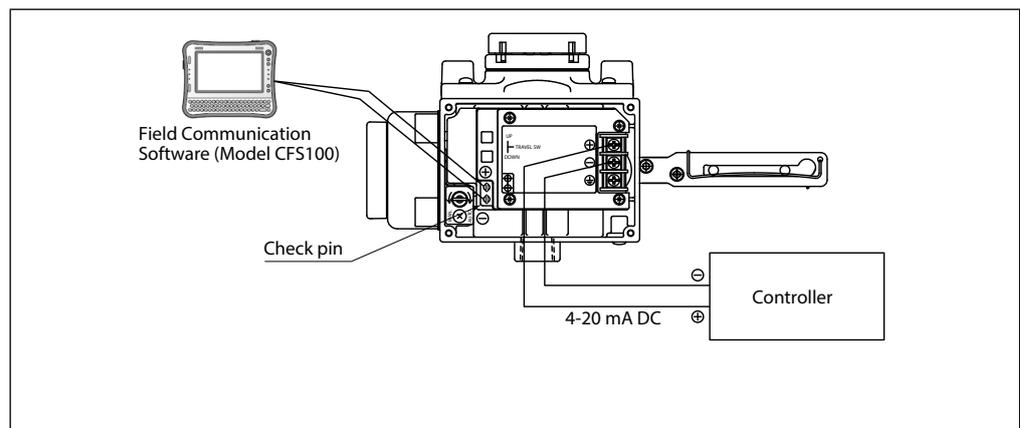
Fig. 4-2. Wiring with Field Communication Software (Model SVX100/102)
