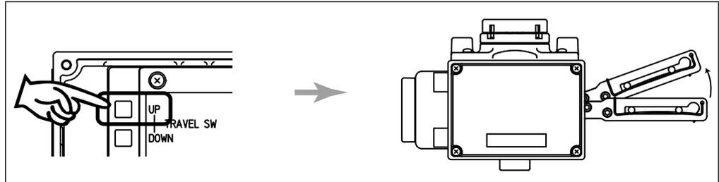
Fig. 3-2. Adjusting the lever in the upward direction
