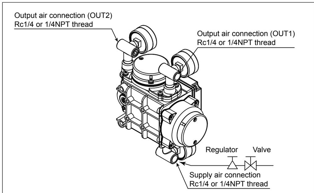
Fig. 2-8. Connecting the air supply (with pressure gauge)
