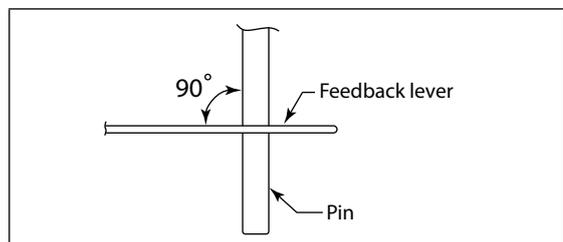
Fig. 2-5. Angle between feedback lever and pin
