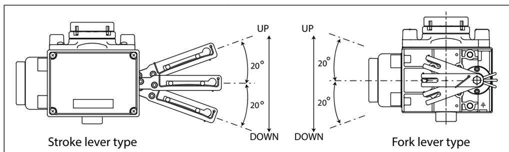
Fig. 2-6. Feedback lever maximum range of motion
