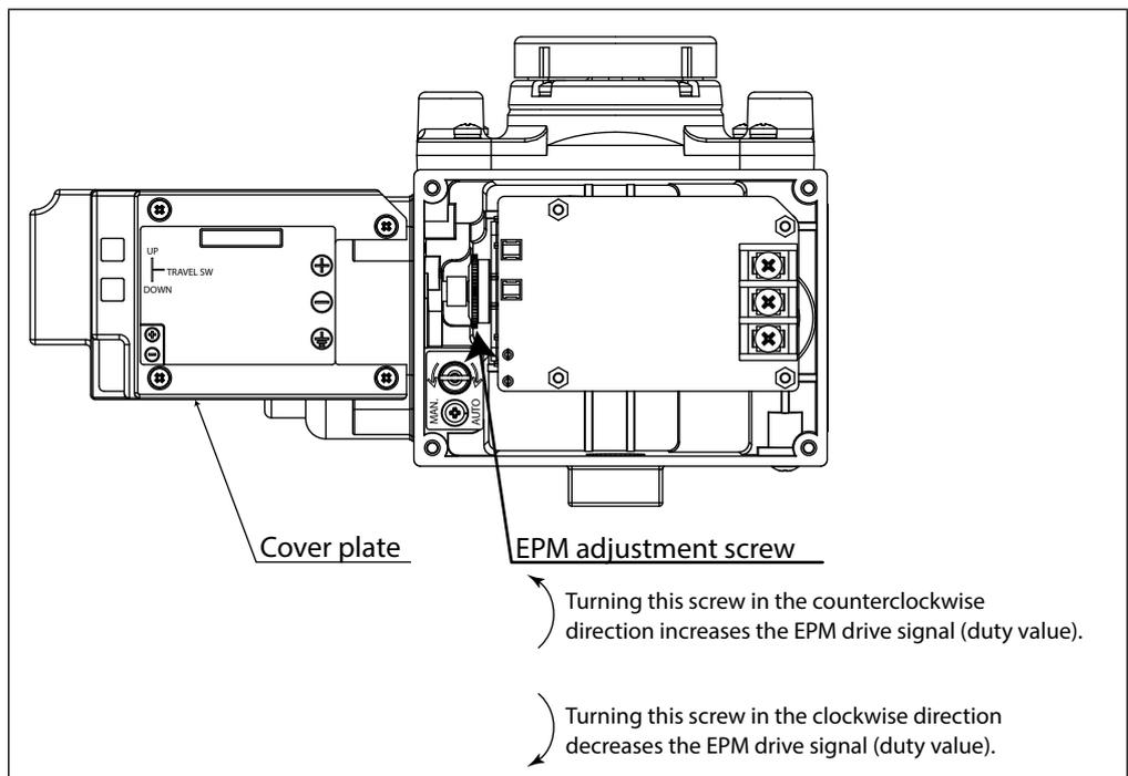
Fig. 5-6. EPM balance adjustment
