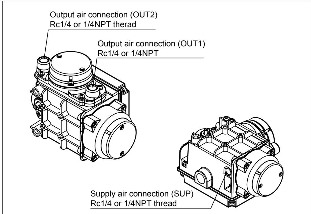
Fig. 2-7. Connecting the air supply (without pressure gauge)
