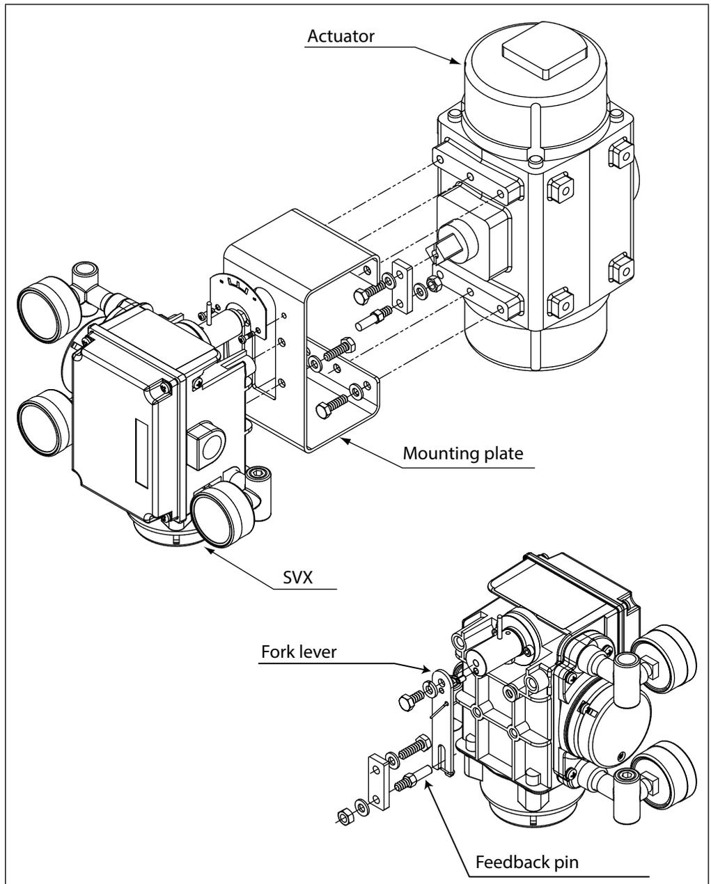
Fig. 2-1. Mounting the rotary cylinder actuator (fork lever type)
