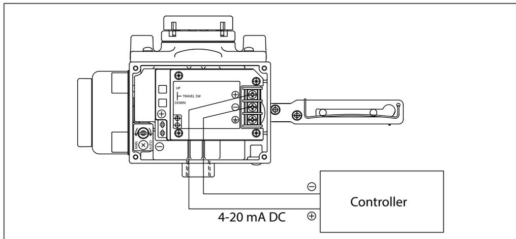
Fig. 2-9. Electrical wiring for model SVX100/102
