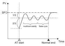
The AT function calculates the PID constants using the limit cycle.
