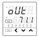
(3) In the MANUAL mode, press the [<], [V], or [^] key to change the MV value.
