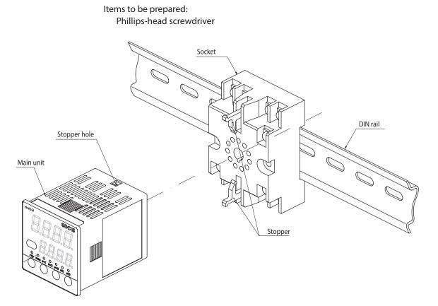
The above Figure shows the DIN rail mounting.
