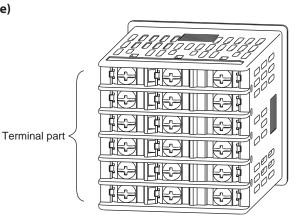
Terminal part: The power supply, input, and output are connected to the terminals. The M3 screw is used. When connecting to the terminal, always use a correct crimp terminal suitable for the M3 screw. The tightening torque of the terminal screw is 0.4 to 0.6 N·m.
