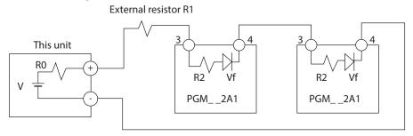
V:  $19 V \pm 15\%$ R0:  $82 \Omega \pm 0.5\%$ R1:  $680 \Omega$ R2:  $260 \Omega$ Vf: 1.1 V
