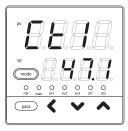
(3) Even though the [<], [V], or [A] key is pressed, the CT input1/2 values cannot be changed.</li>
