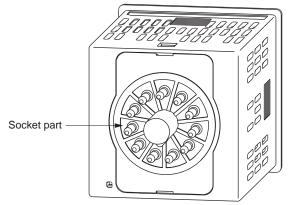
Socket part: This socket is inserted into the optional socket. The power supply,
