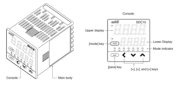
Main unit: Contains the electric circuit for I/O signals of measuring instruments, CPU, and memory.
