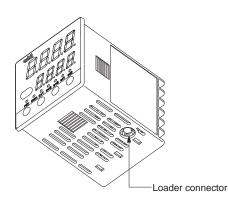
Loader connector: This connector is connected to a personal computer using the dedicated cable supplied with the Smart Loader Package.
