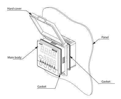
Both gaskets must be used, one is supplied with the main unit and the other is supplied with the hard cover. Both are the same gaskets.
