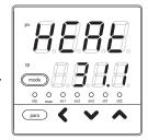
(3) Even though the [<], [V], or  $[\Lambda]$  key is pressed, the heat MV and cool MV cannot be changed.
