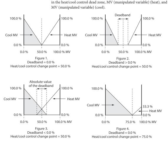
For details, refer to Single Loop Controller Model C15 User's Manual "Installation & Configurations" (CP-SP-1148E 13th edition or later)
