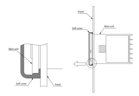
The gasket supplied with the main unit is not used.
