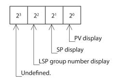
• When using the SLP-C35 Smart Loader Package, not only the numeric value, but also the bit input can be used to set [274: PV/SP display setup].
