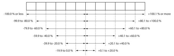
Lighting range of deviation graph (Ratio of deviation (PV-SP) to Multi Status (MS) display deviation range)
