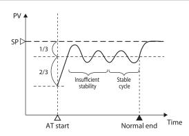
In the Heat/Cool control, the AT function is run in the status that both the heat MV and cool MV are operated.
