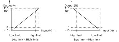
However, the output is 0 to 110 % in a range of 0 to 20 mA.
