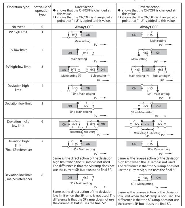
\* If the setting is made so that the main setting is greater than the sub setting, the operation is performed with the main setting swapped for the sub setting automatically.
