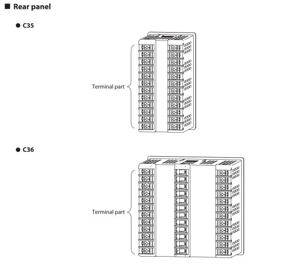
Terminal part: The power supply, input, and output are connected to the terminals. The M3 screw is used. When connecting to the terminal, always use a correct crimp type terminal lug suitable for the M3 screw. The tightening torque of the terminal screw is 0.4 to 0.6 N·m.
