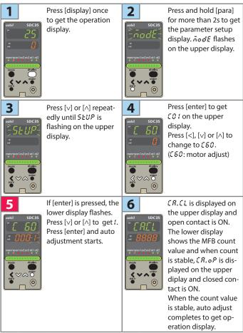
After starting auto adjust, press [display] key to stop auto adjust. During auto adjust the key operation except [display] key of stopping auto adjust is impossible.
