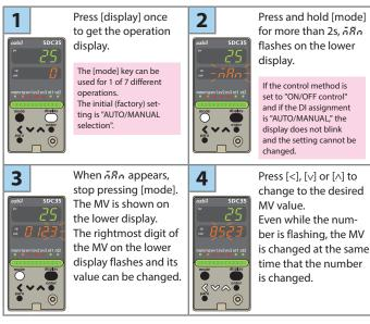
For the flashing MV in step 3, either bumpless transition (the same value as before the change) or preset MANUAL value (the value set in setup  $\mathcal{LO}$ ) can be selected (in setup  $\mathcal{LO}$ , Output operation at changing Auto/Manual).
