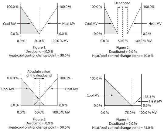
In figure 4, when the MV is 100 %, the heat MV is 33.3 %. In this case, when the heat/cool control change point is 50 % or more, if the MV is 100 %, the heat MV high limit is less than 100 %. The change rate of the heat MV relative to the MV is the same as that of the cool MV relative to the MV.
