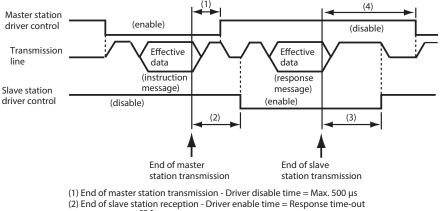
setup setting (270) or greater (3) End of slave station transmission - Driver disable time = Max. 10 ms
