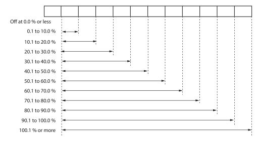
• When the lighting status is set at "9" (MV graph), "10" (Heat-side MV graph), "11" (Cool-side MV graph), or "12" (MFB graph), the Multi Status (MS) display is lit as shown in the following Figure:
