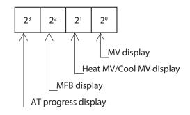
• When using the SLP-C35 Smart Loader Package, not only the numeric value, but also the bit input can be used to set [£75: MV display setup].
