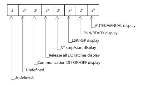
• When using the SLP-C35 Smart Loader Package, not only the numeric value, but also the bit input can be used to set [C73: MODE display setup].
