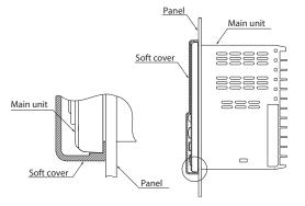
The gasket supplied with the main unit is not used.
