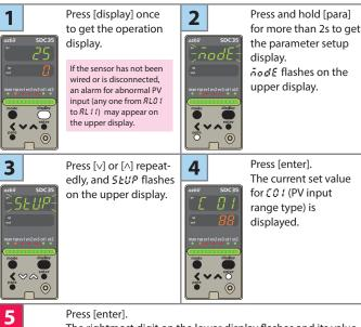
The rightmost digit on the lower display flashes and its value can be changed.
