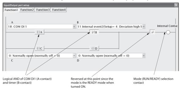
DI Assignment (Internal Contact 2): Input/Output port setup
