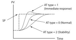
The following figure shows the conceptual diagram expressing differences in control result using the PID constant calculated by each AT type:
