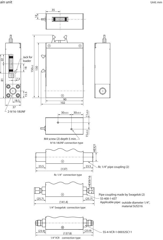
Model with separate display MQV0050K/0200K/0500K
