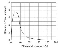
Relationship between differential pressure and outlet flow rate when valve of MQV0500 is fully closed (air flow under conditions of outlet pressure = 0 kPa (gauge))
