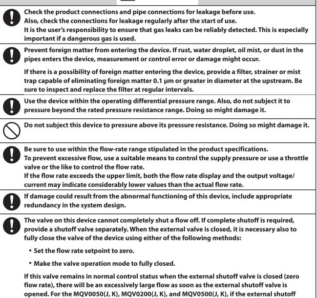
opened. For the MQV0050(J, K), MQV0200(J, K), and MQV0500(J, K), if the external shutoff valve is closed continuously for 5 minutes or more in control mode or with the valve forced fully open, the valve overheating limit (AL71) will be activated and the current to the valve will be forcibly limited.
