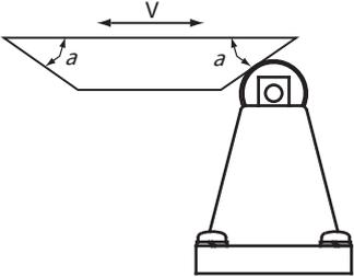
When using with the dog speed (V) faster than 0.3 m/s, change the dog angle ( $\alpha$ ) according to the table below.
