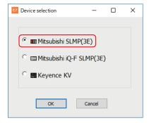
PLCLink Common Transfer 1 Transfer 2 Transfer 3 Transfer 4 IP address 192 . 168 . 0 . 1 Mitsubishi SLMP(3E) Device selection 1025 Port Retry 1000 TimeOut(ms) SendDelayTime(ms) Cyclic transfer scan cycle(ms) 200 Triggered transfer scan cycle(ms) 500 Startup delay time (s) Trigger device initialization
