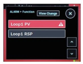
On the function alarm screen, the alarm status is distinguished by color for each function.
