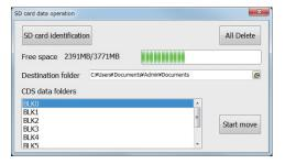
Clicking the [SD card identification] button displays the available space on the microSD memory card and the CDS data folders.
