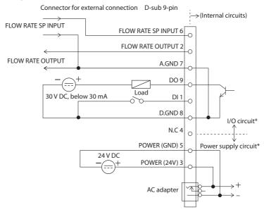
\* The power supply circuit and I/O circuit are isolated.
