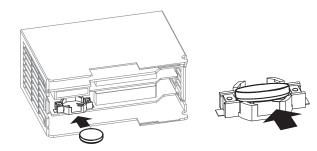
(2) Press the battery with your finger to set it in place on the battery holder.
