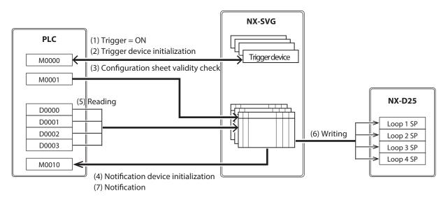
The NX-SVG executes triggered data transmission as shown below.
