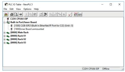
(2) Double-click "CJ2B-EIP21 (Built-in EtherNet IP/Port for CJ2)."
