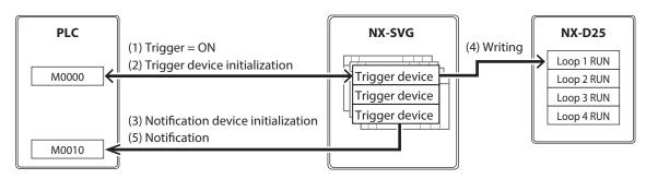
(1) According to the cycle set by [Common: Trigger Scan], the NX-SVG reads the Trigger(Write OFF) and Trigger(Write ON) devices set in the rows on the configuration sheet to monitor whether they turn from OFF to ON. When the trigger device turns on, the NX-SVG starts to process bit setting. The trigger device scan cycle and trigger detection timing are the same as for triggered data transmission.
