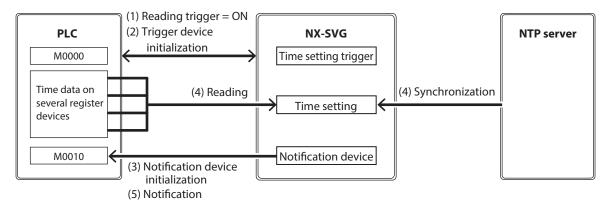
(1) According to the cycle set by [Common: Trigger Scan], the NX-SVG reads the time setting trigger device to monitor whether the device turns from OFF to ON. When the trigger device is turned on, time setting starts. The trigger device scan cycle and trigger detection timing are the same as for triggered data transmission.
