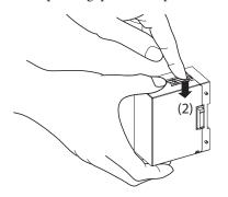
(3) While pressing the tip of the lever, rotate the main unit down to remove it.
