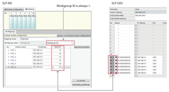
In the mapping table of the SLP-NX, set the device numbers assigned by the SLP-SVG for the node IDs of the Network Instrumentation Modules.
