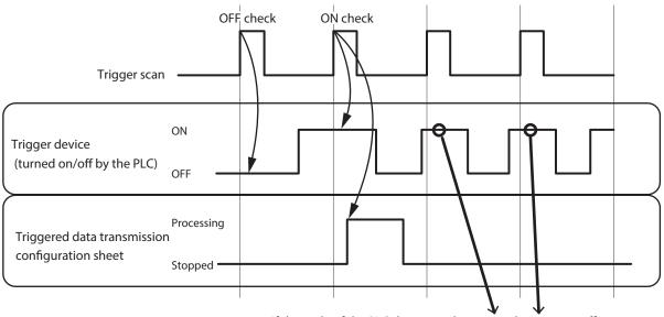
If the cycle of the PLC that turns the trigger device on or off is much faster than the trigger scan cycle, the trigger cannot be detected.
