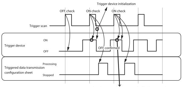
When the trigger device is turned off by the trigger device initialization function, the next trigger will be detected.
