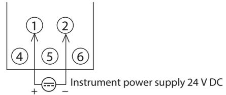
The power supply unit must be a UL Class 2 power supply unit.
