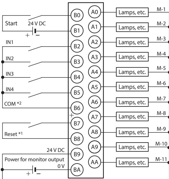
\*1. Use the reset input by itself. It cannot be used together with another RX-R40/20 reset input.
