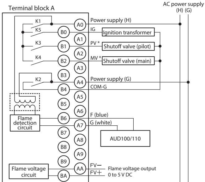
\* If you select the direct ignition method in the SLP-RX, connect the main burner safety shutoff valve to terminal(B1).
