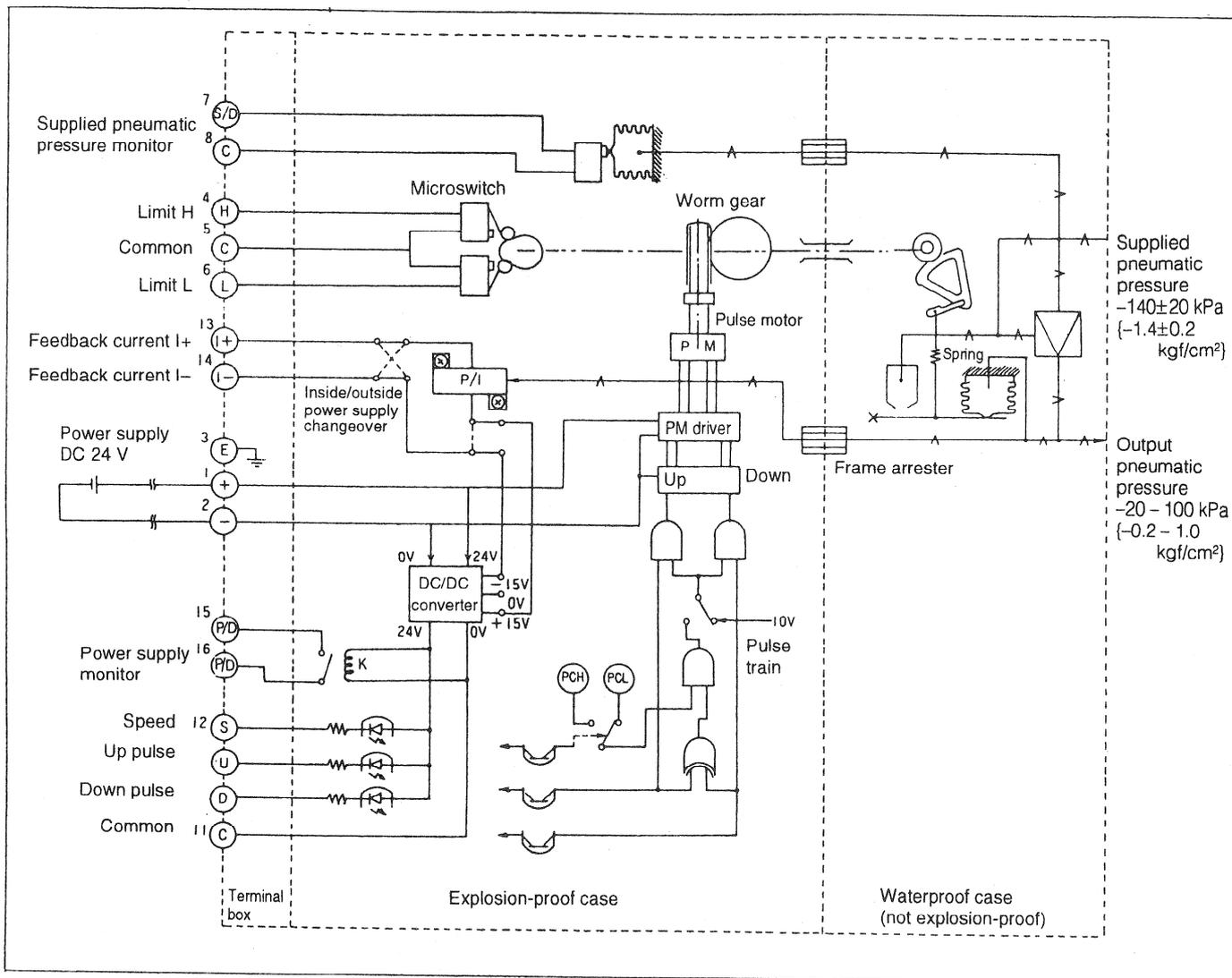
Figure 4-1 Block diagram
