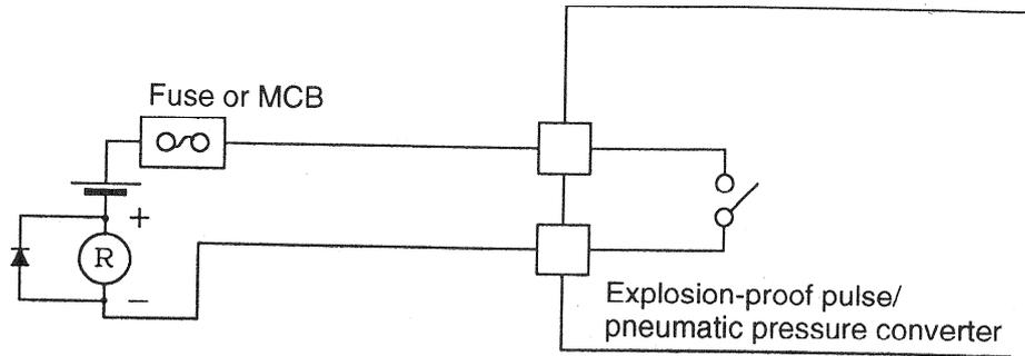
For safety, combine the converter with a surge suppression device on the load side of contact output.
