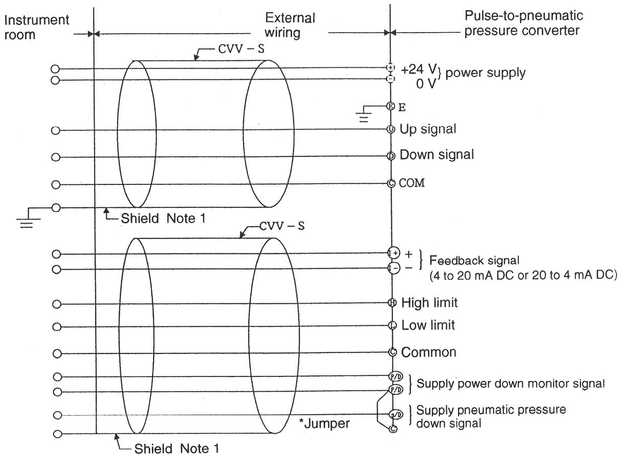
**Note 1:** Ground the cable shield only on the instrument room (Class 3 or higher).
