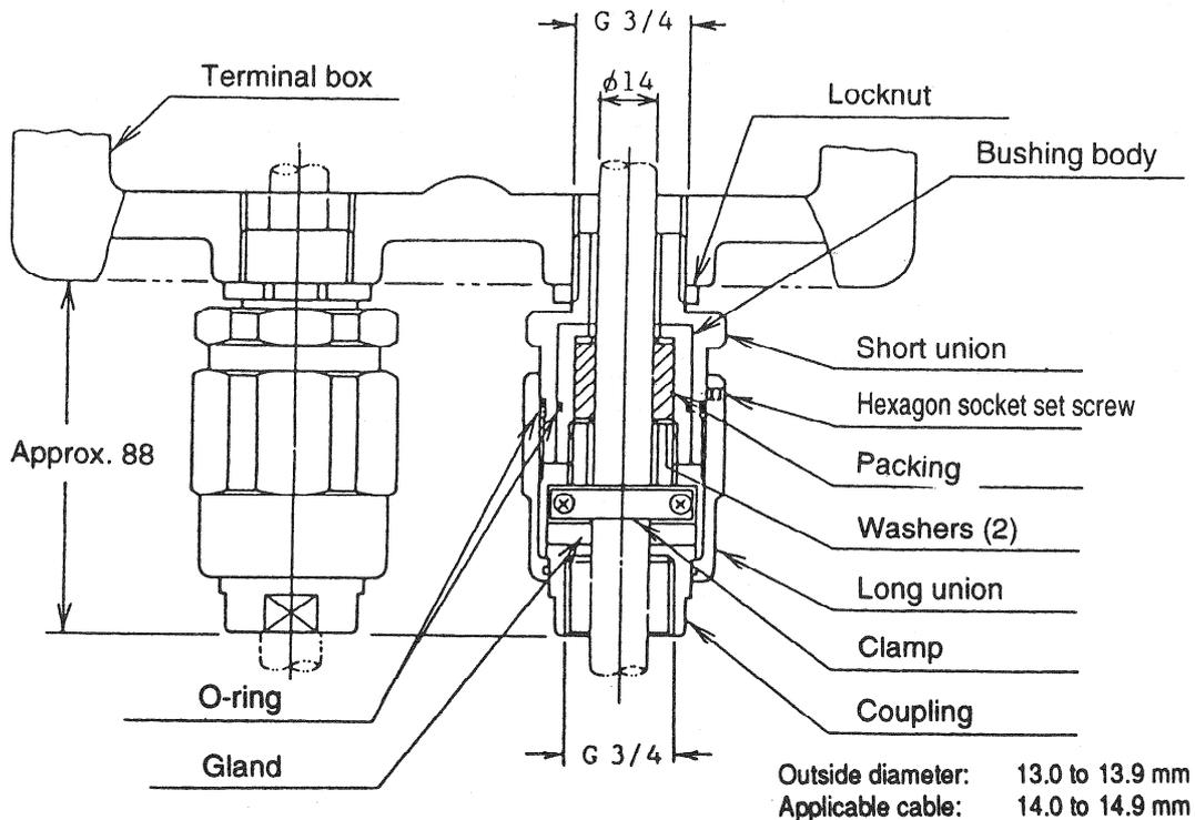
Figure 5-4 With cable adapter with pressure resistant packing
