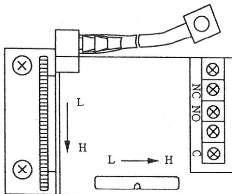
Figure 6-3 Pneumatic pressure monitor unit
