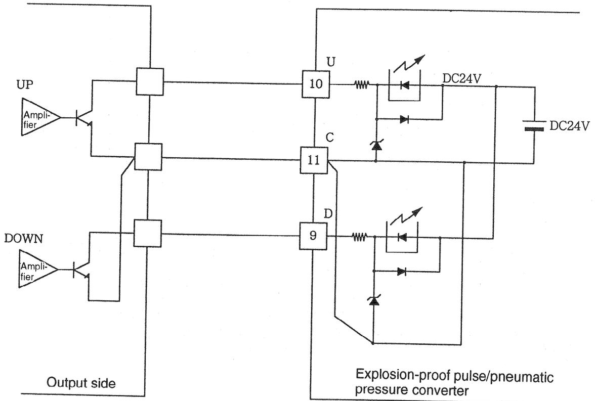
Open collector output is desirable for up/down signals.
