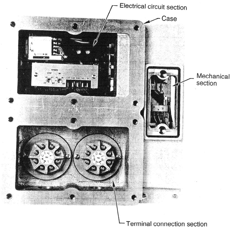
Figure 4-2 Converter configuration and names of parts
